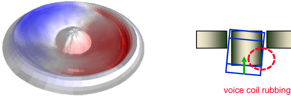
Figure 13: Rocking mode (left) and voice coil rubbing (right)
