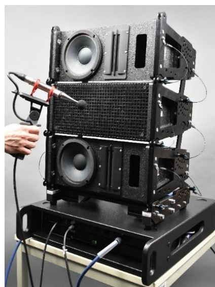
Figure 3: Fast and cost-efficient quality check of rental Sound Reinforcement Equipment using streaming V/I amplifiers and QC Stand-alone Software.
