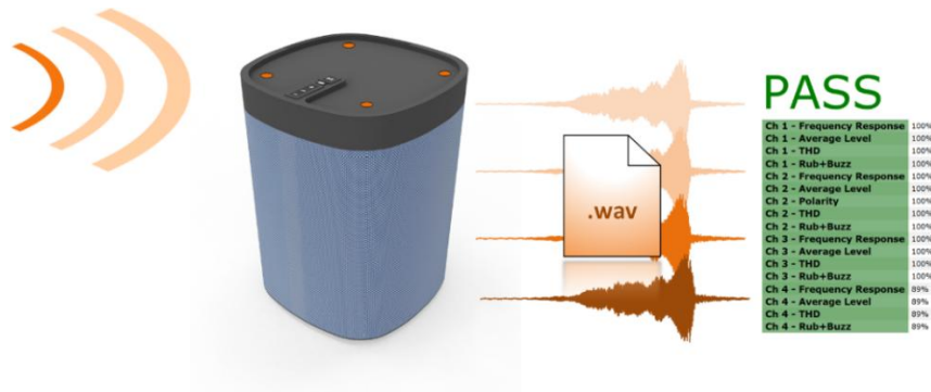
Figure 15: Wave file-based testing a smart speaker's four microphone responses using KLIPPEL QC.
