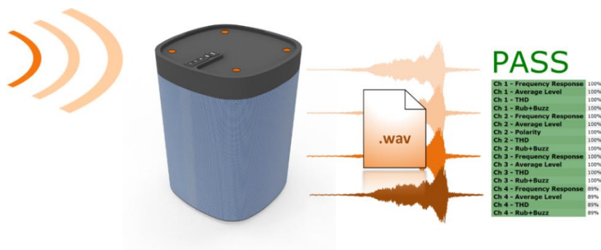
Figure 16: Wave file-based testing a smart speaker's four microphone responses using KLIPPEL QC.
