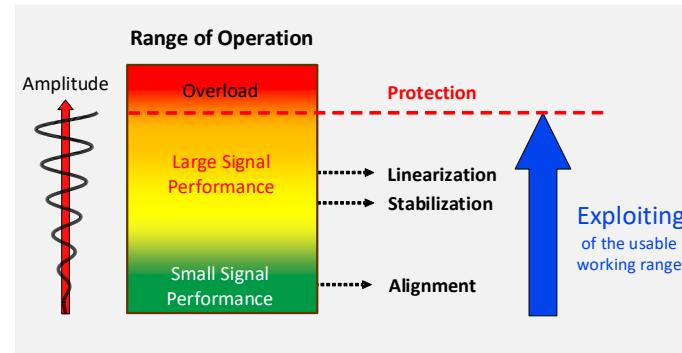
Loudspeakers are highly nonlinear and time-variant systems. Signal distortion, heating, aging, climate and other external influences limit the maximum level and the quality of the reproduced sound. The adaptive nonlinear control system KCS can cope with these undesired effects and generate the desired linear behavior over the entire working range.
