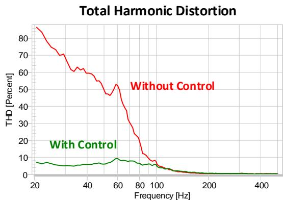
The harmonic and intermodulation distortions synthesized in the mirror filter are subtracted from the input signal before it is fed to the transducer. Thus, the distortions generated by the transducer are compensated, and a linear relationship between the input signal and sound pressure output at any point in the sound field is established.
