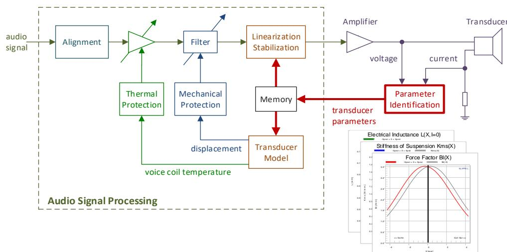
While playing music in on-line mode, KCS constantly monitors voltage and current at the speaker terminals to continuously adapt the internal model with time varying transducer properties, such as variances of mechanical stiffness, voice coil temperature and voice coil position. Based on the identified parameters, the nonlinear transducer model estimates precise state information such as voice coil displacement, which is required by the protection systems.
