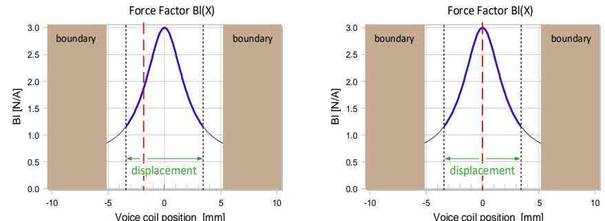
KCS detects the absolute position of the coil without a mechanical sensor by monitoring the input current and identifying an offset in the nonlinear curves. The detected offset can be actively compensated by supplying an appropriate DC voltage to the transducer via a DC-coupled amplifier. This ensures maximum positive and negative voice coil swing, giving maximum bass generated at high efficiency over the lifetime of the speaker.
